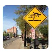
Special signs are posted along the streetcar route to remind cyclists about the track gap, particularly when turning corners onto the streetcar route.
