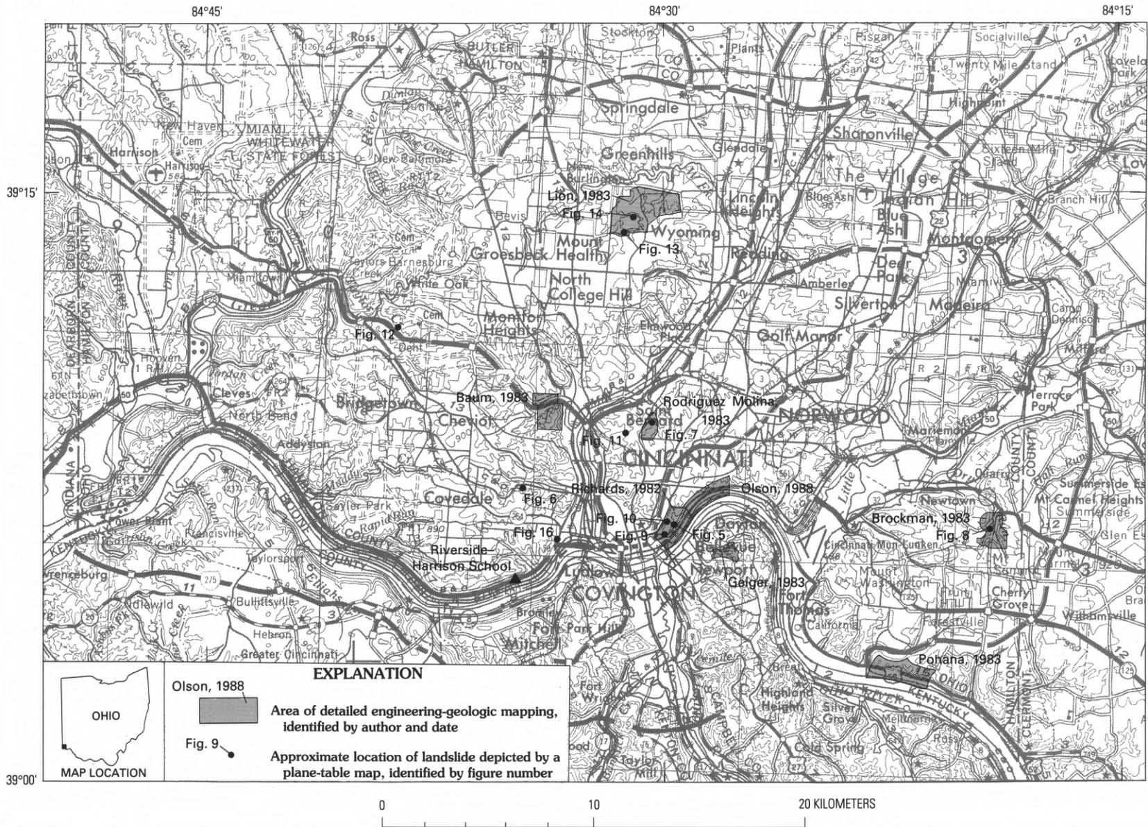
**Figure 1.** Map of Cincinnati and Hamilton County, Ohio, showing approximate outlines of areas of detailed engineering-geologic mapping by students at the University of Cincinnati and locations of landslides depicted by plane table maps. Base from U.S. Geological Survey 1:250,000 Cincinnati, Ohio; Indiana; Kentucky (1953, revised 1974). Contour interval 100 feet.
